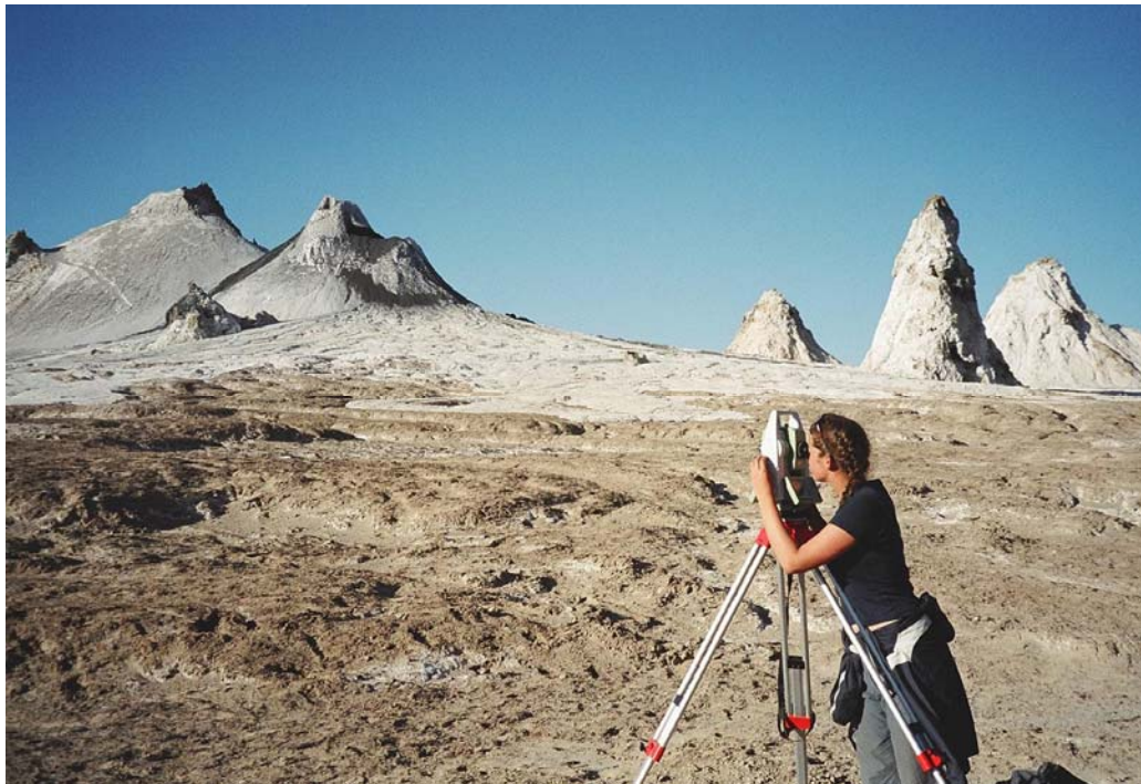
Recording points to model the Ol Doinyo Lengai crater using the Leica TPS1200 Total Station with reflectorless EDM
